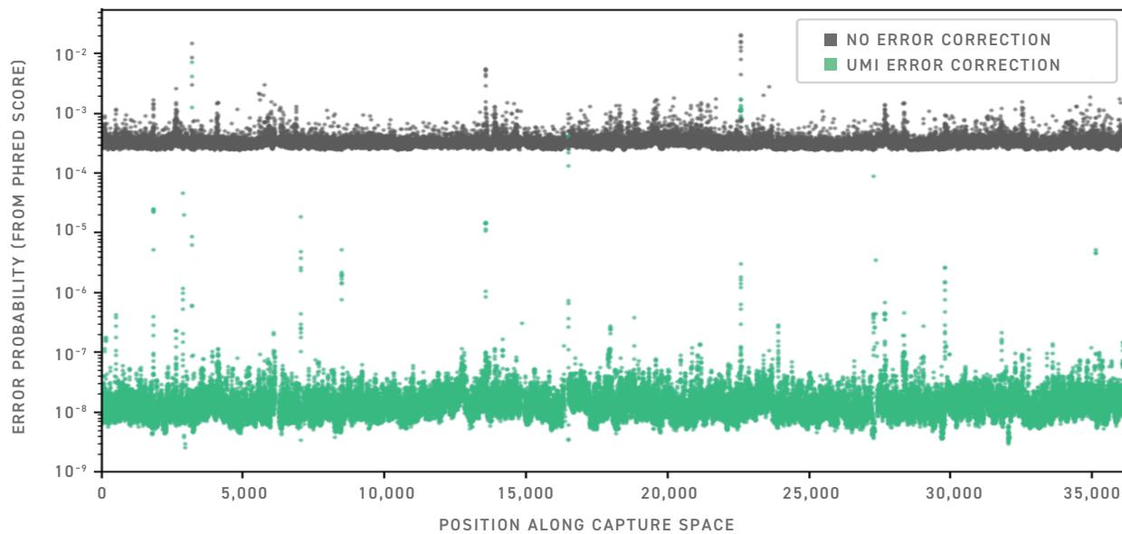
Estimated per-base error rate for non-error-corrected reads (gray) and error-corrected reads (green) measured from target enrichment of a synthetic cfDNA standard. After sequencing, reads were downsampled to 20,000x coverage and error correction was performed using duplex collapse, requiring at least one read from each original strand.
