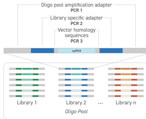
CLUE Oligo Pool design. Each library within the pool is assigned a specific adaptor which can be used for PCR amplification of that specific library. NGS-based quality assessment of 10 pooled sgRNA libraries produced from a single oligo pool.
